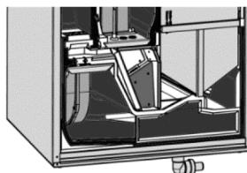
3. Remove any deposits from the condensation tank and/or the drain line. Flush the line out with sufficient water.
