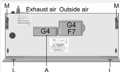
Tilt front plate forwards at the two top corners (magnets [M]) and remove from above. Remove filter cover [A].
