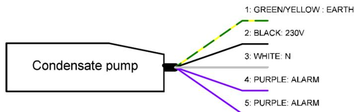
The condensate pump contains an internal sensor that will automatically start the pump when the water level rises above approx. 15 mm and stop the pump when the water level has fallen to approx. 5 mm. The condensate pump is also fitted with a high water level alarm that will operate the alarm relay if the water level rises above approx. 25 mm. The pump will continue to run until the minimum water level is reached and the alarm will reset.
